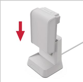
Plug in the charger. Attach the battery pack to the charger by aligning the ribs on the battery pack to the grooves in the charger.
