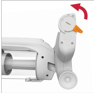
Turn the tab on the brushbar cover anticlockwise to release the brushbar.
