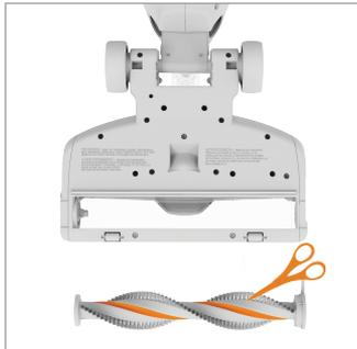
To remove any threads or hair, slide the blade of a pair of scissors into the groove on the brushbar and cut along the groove.
